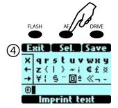
Use the front and rear wheel to find the Copyright sign. This is located low down on the list, so you will have to scroll down a few screens to find it. (11 times down with the rear wheel and 5 times to the right with the front wheel). Now press "Sel" button to select the © character.
