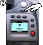
Use the front wheel to select the menu "Settings", then press the "Drive" button. (marked with "Enter" on the LCD)
